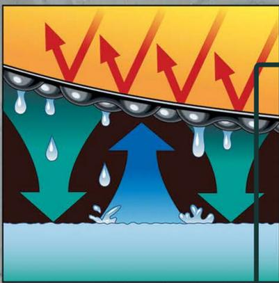
EvapGuard<sup>TM</sup> material provides evaporation control, algae inhibition, debris reduction and temperature regulation. The material can be applied in modular sections or as a complete covering membrane to the surface of the water. With the addition of small holes during the fabrication process the cover can also be used for rain water harvesting.
