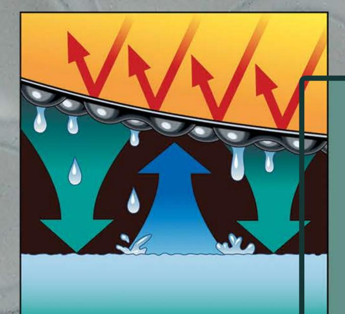
EvapGuard™ material provides evaporation control, algae inhibition, debris reduction and temperature regulation. The material can be applied in modular sections or as a complete covering membrane to the surface of the water. With the addition of small holes during the fabrication process the cover can also be used for rain water harvesting.
