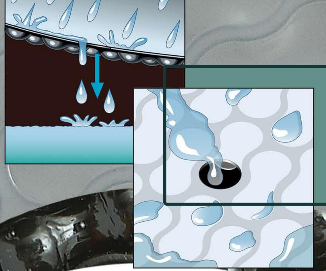
The addition of holes in the cover means that the EvapGuard™ material can help to harvest water, while also reducing evaporation.
